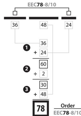
7. Modular wiring components. Internal panel wiring is fully modular and is field-installed into the raceway of panels. When wiring is field-installed the following components must be specified:
